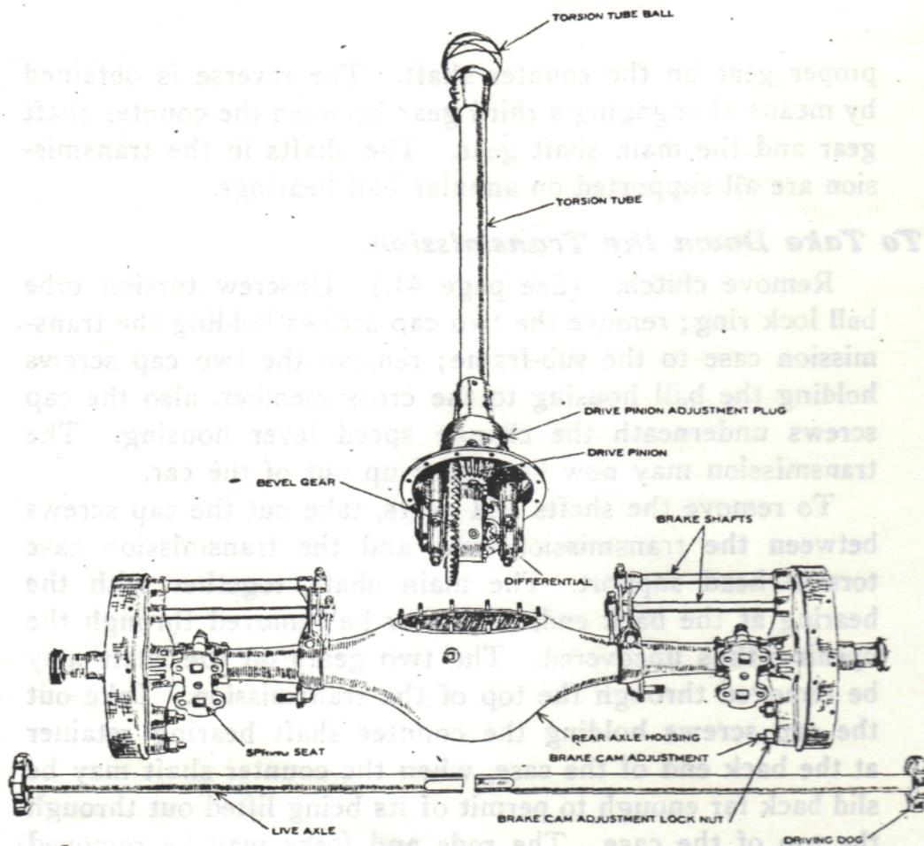
ting power. The brakes are both of the internal expanding type and are operated in dust protected drums by means of cams.
