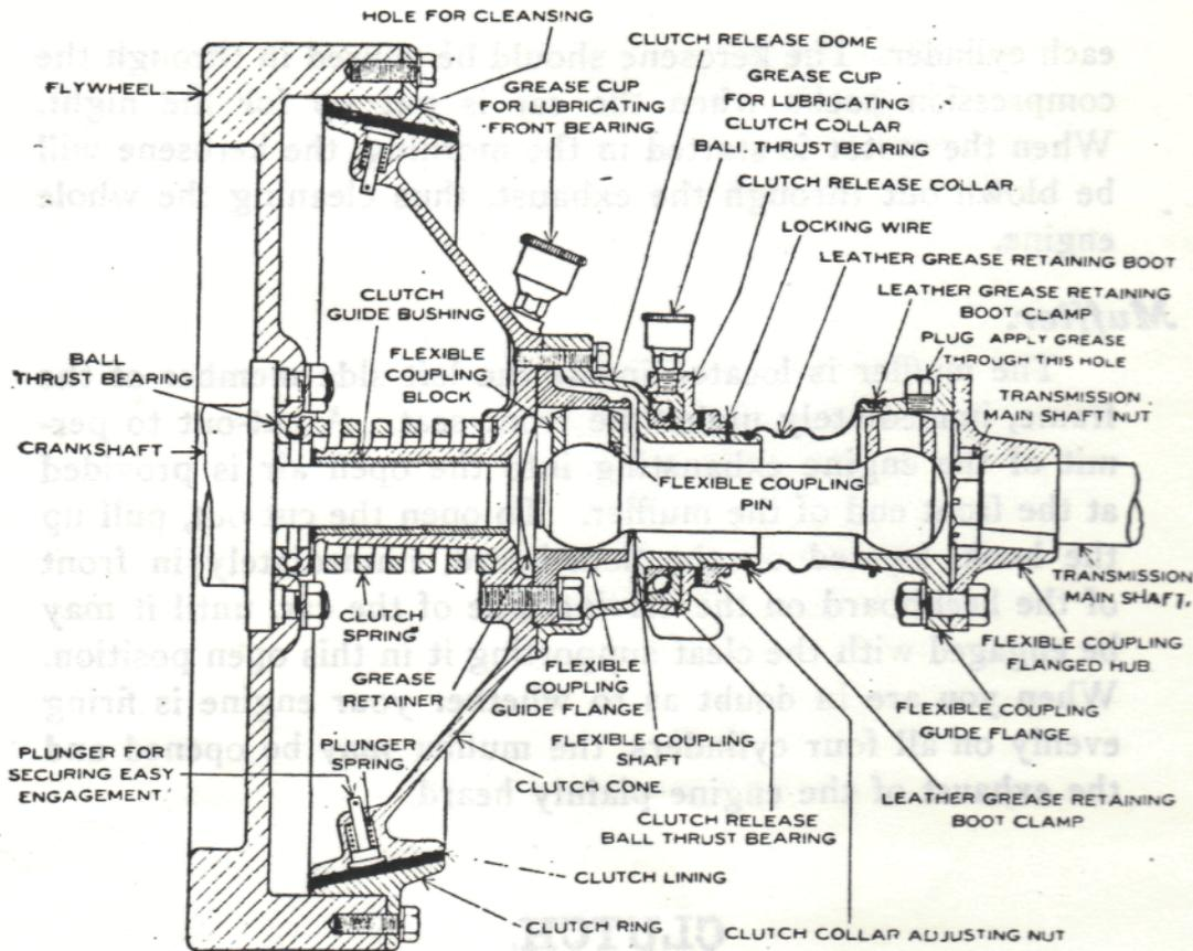
Cross Section Through Clutch.
