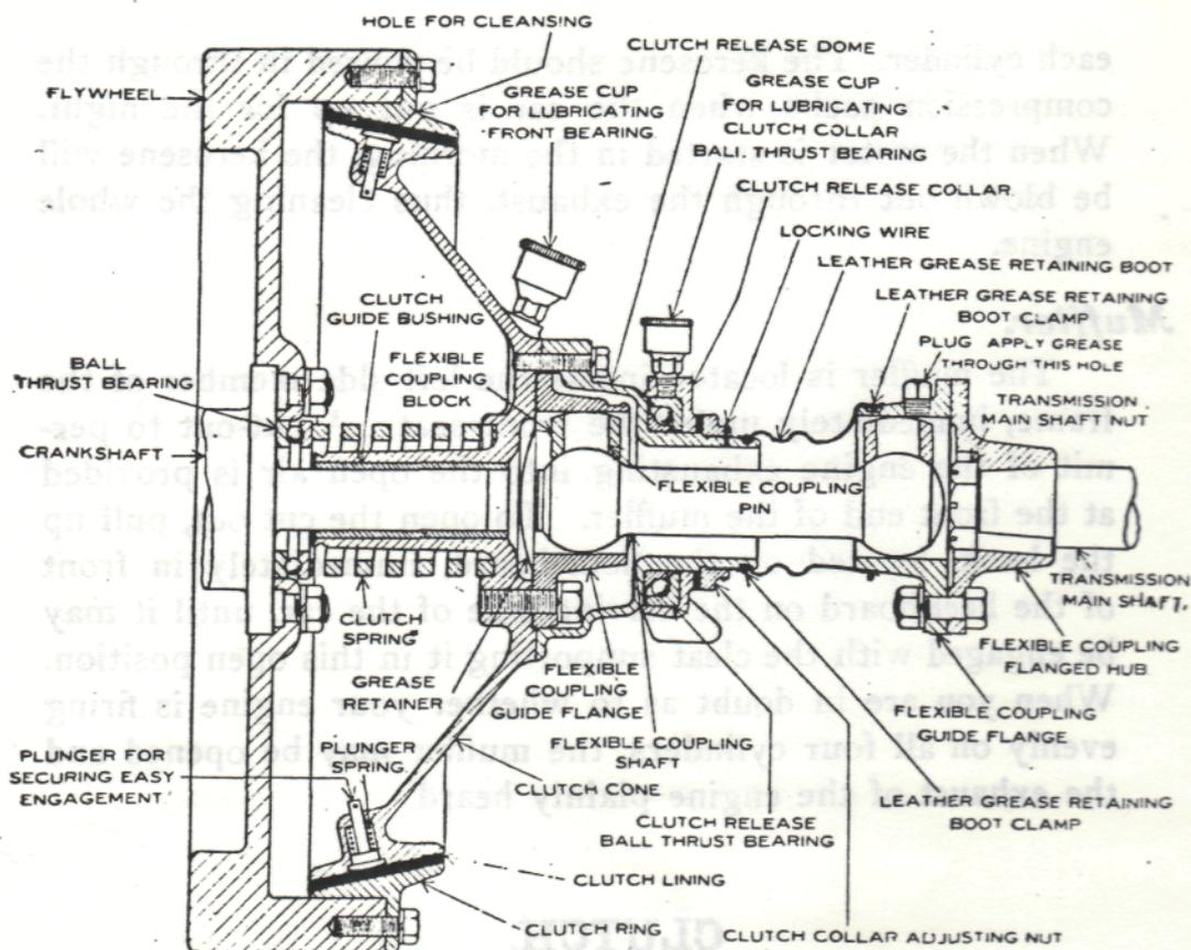
Cross Section Through Clutch.
