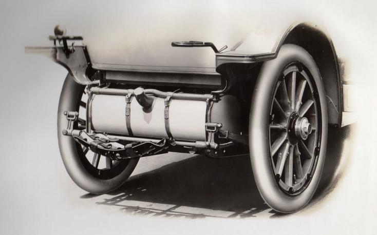
THE "AMERICAN TRAVELER" TANK Details of the tire-holders, tank rack, etc.
