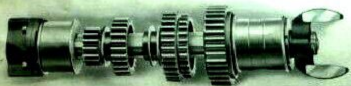
Primary Shaft with Gears, Bearings, Bearing Retainers and Universal Joint which is Part of Universal Coupling at the Rear of Transmission
